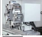
Hydraulic turret H4-VDI Hydraulic turret V8,V12
